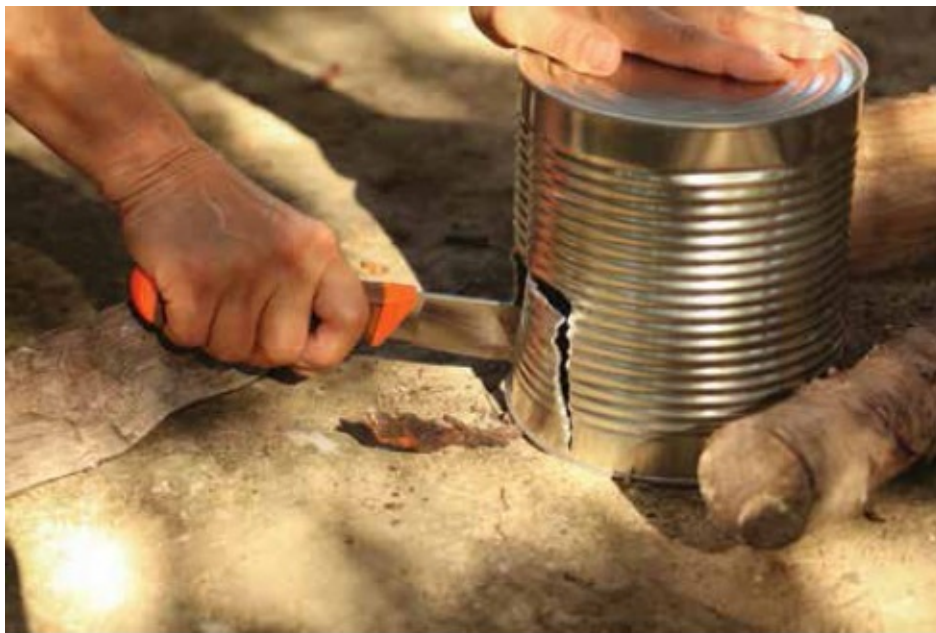
Making a hobo stove from a #10 can with an OKC Cayuga Hunter © JAYRES
