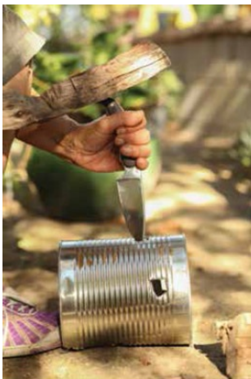
Cutting air holes into can for hobo stove © JAYRES
